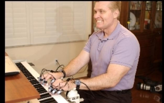
*An adjustable stand connected to a track with two wrist pilots, two sets of finger signal sleeves, two motors, controller and a power supply. A laptop computer is running the Concert Hands software program.*
